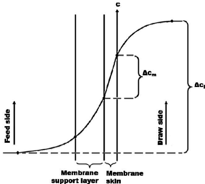
Figure 6. Concentration polarization causes the effective concentration difference  $\Delta c_m$  to be only a fraction of the bulk concentration difference  $\Delta c_b$ .
