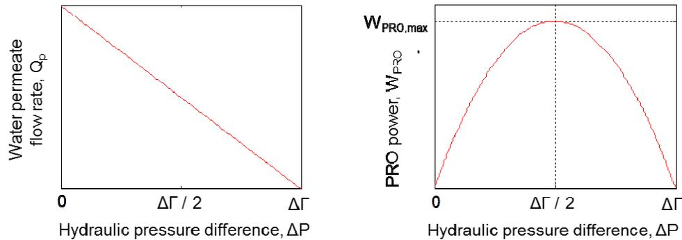
**Figure 2. Water permeate  $Q_p$  and PRO power  $W_{PRO}$  as functions of the hydraulic pressure difference  $\Delta P$ . The maximum power point  $W_{PRO,max}$  is obtained when  $\Delta P = \Delta \Gamma / 2$ .**
