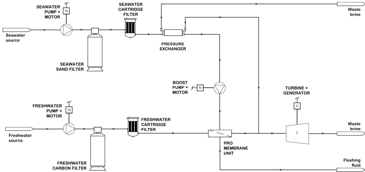
Figure 3. Diagram of PRO power plant prototype.
