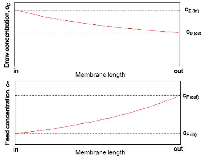
Figure 5. Variation in feed and draw concentrations along the length of the membrane.
