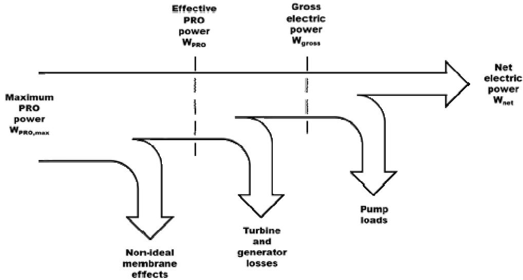
Figure 4. Power flow in a PRO power conversion system.
