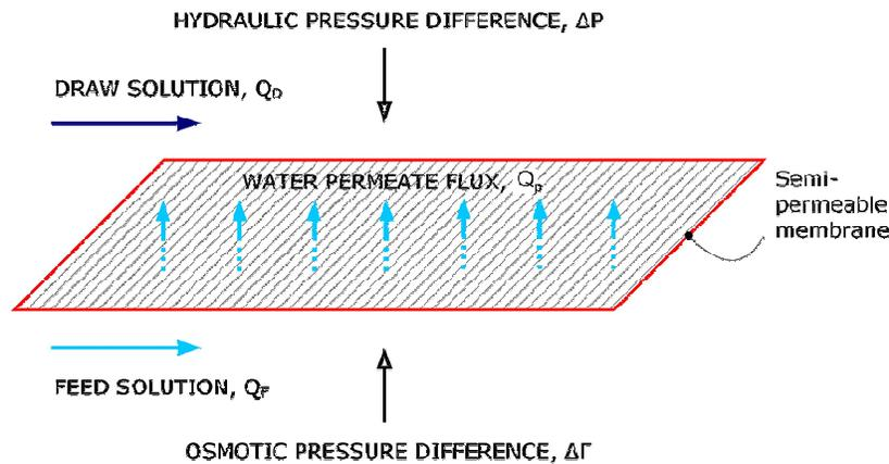
**Figure 1. The process of pressure retarded osmosis (PRO).**
