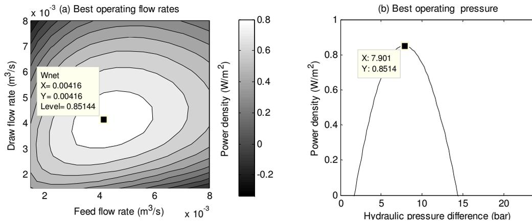
**Figure 7. Operating conditions for achieving maximum net electric power output, showing the best feed and draw supply flow rates, and the best hydraulic pressure difference across the membrane.**
