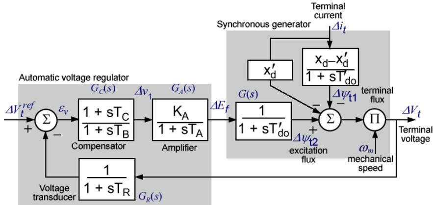
Figure 3 Diesel genset electric subsystem structure
