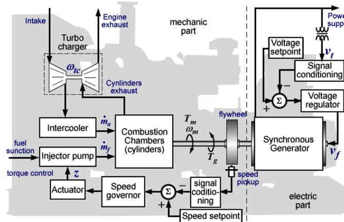
**Figure 1. Diesel generator set block diagram.**
