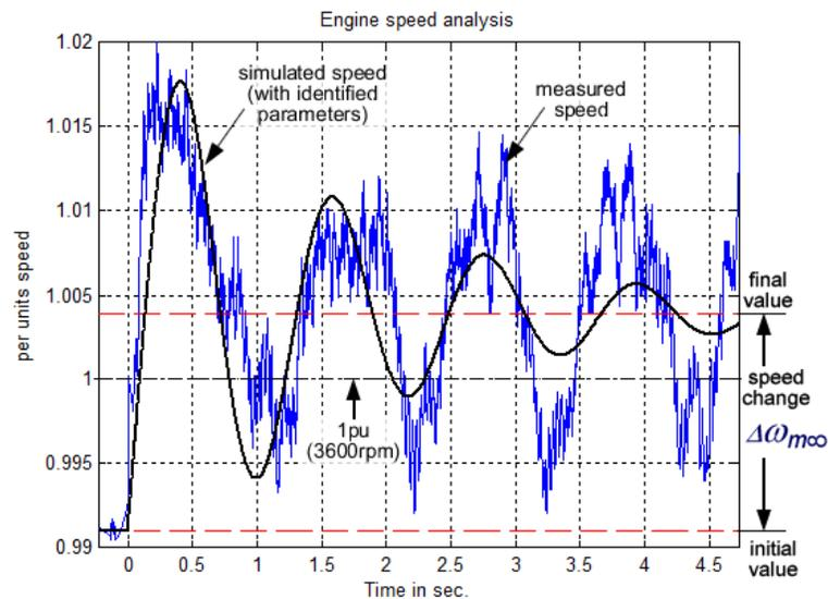
**Figure 6. Speed transient following a purely resistive load rejection test**
