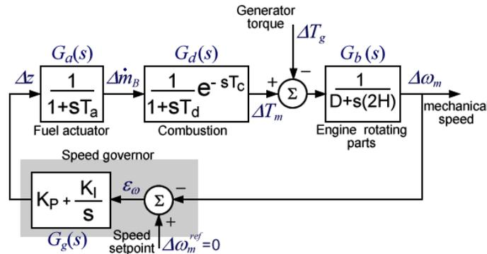
**Figure 2. Diesel genset mechanical subsystem structure**
