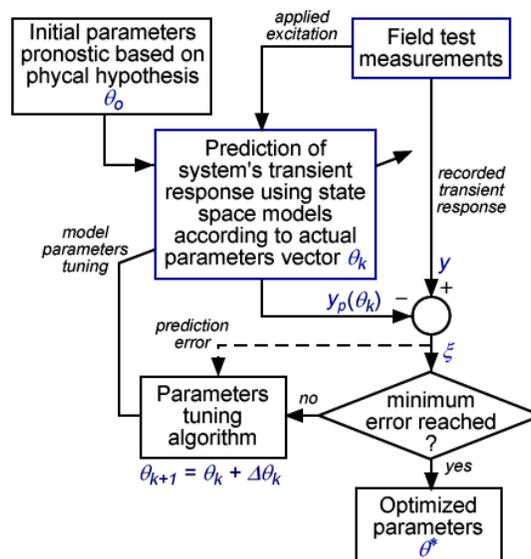
Figure 4. Flowchart for the parameters identification loop (based on [16])
