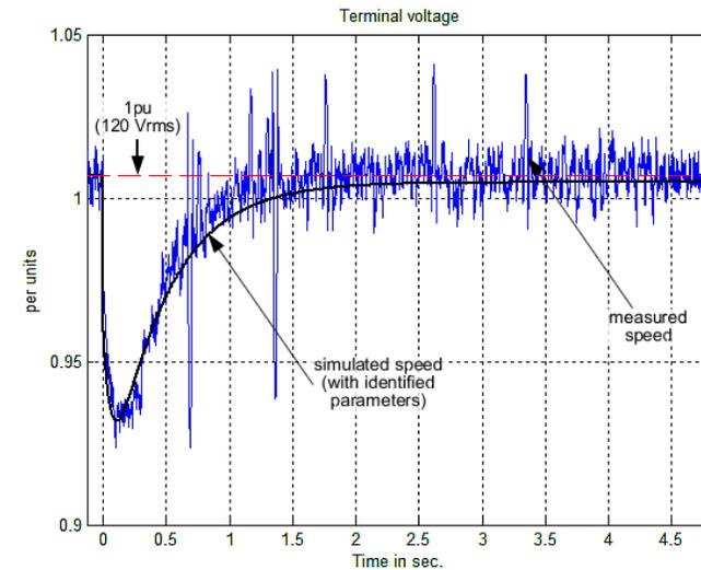
**Figure 7. Terminal Voltage transient following a purely capacitive load rejection test**
