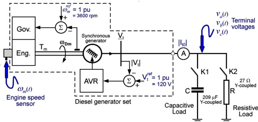
**Figure 5. Experimental setup schematic diagram**
