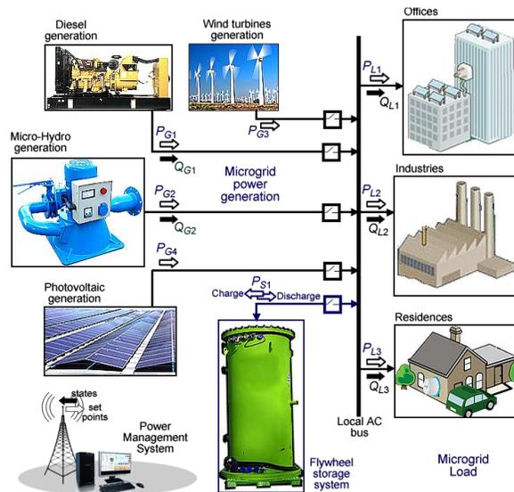
Figure 1. Microgrid system main components
