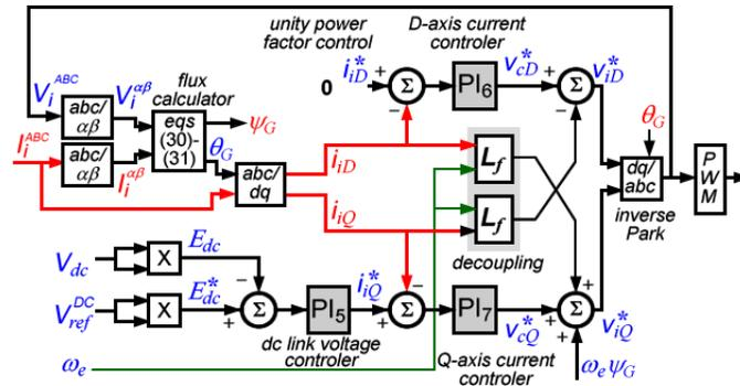
Figure 6. Motor side converter control scheme
