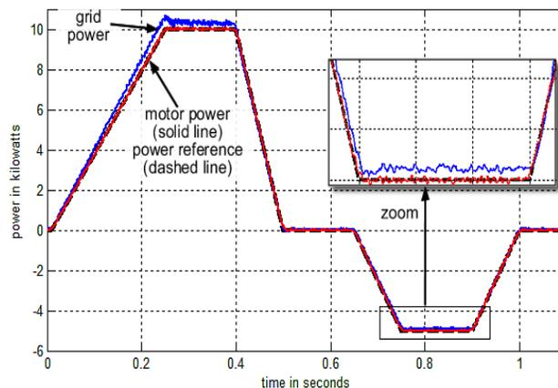
**Figure 7. Power comparisons of the flywheel storage system**
