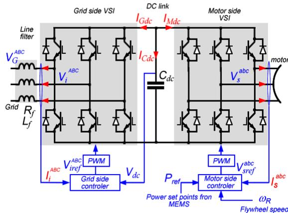
**Figure 4. The back-to-back power converter**
