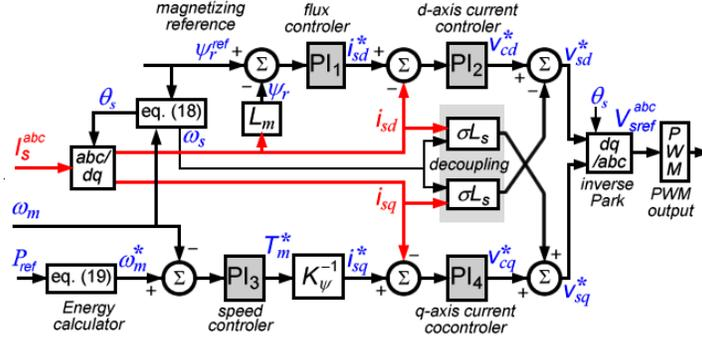
**Figure 5. Motor side converter control scheme**
