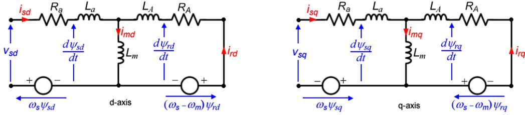
**Figure 3. Induction machine equivalent circuit in the dq-frame**
