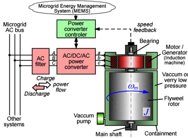
**Figure 2. Flywheel energy storage system structure**
