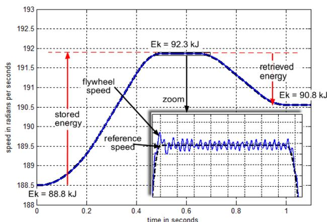
Figure 8. Comparisons between flywheel speed with the reference speed
