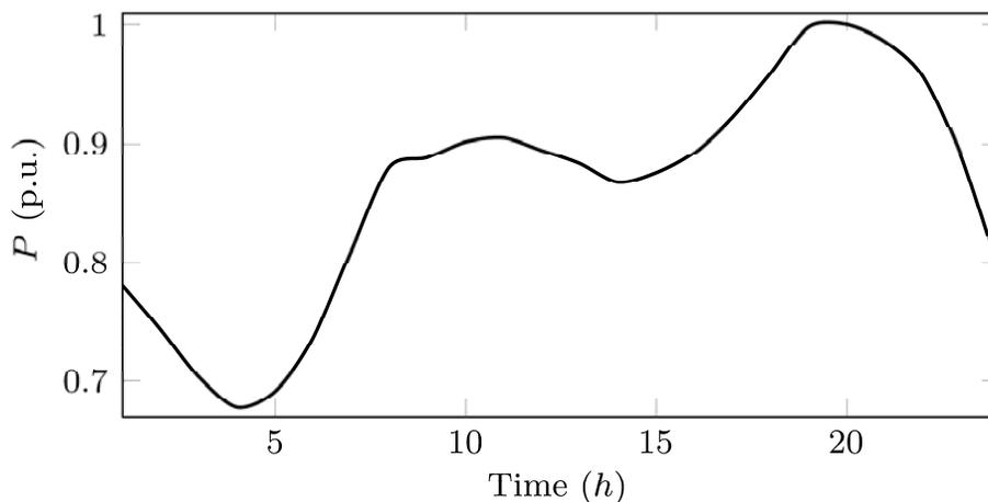
**Figure 5. Daily load curve for the test system.**
