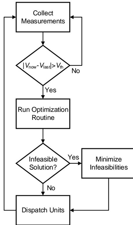
Figure 3. Closed-loop Volt-VAR control algorithm for near-real-time.
