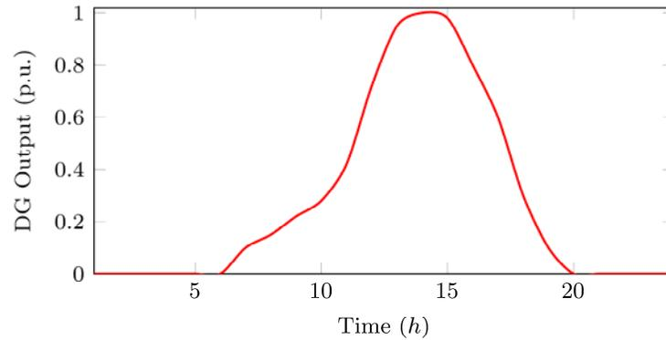
Figure 6. Daily generation curve for DGs (photovoltaic system).
