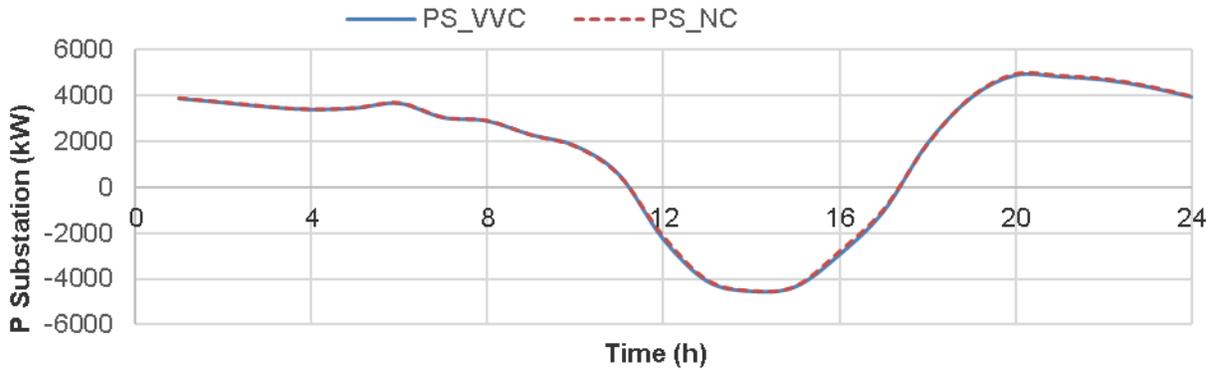
Figure 10. Total active power injection by the substation for “No Control” and “VVC” cases.
