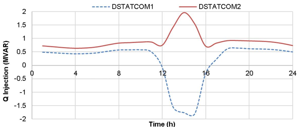
Figure 12. DSTATCOMs output obtained using VVC algorithm.
