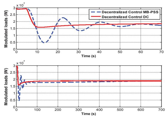
**Figure 12. Modulated MW with decentralized control and no reserve/80 MW spinning reserves**
