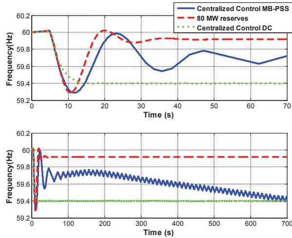
**Figure 8. System frequency of centralized control with no reserve/80 MW spinning reserves**
