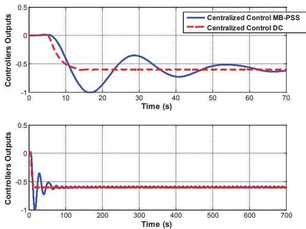
**Figure 9. Controllers outputs with centralized control and no reserve/80 MW spinning reserves**
