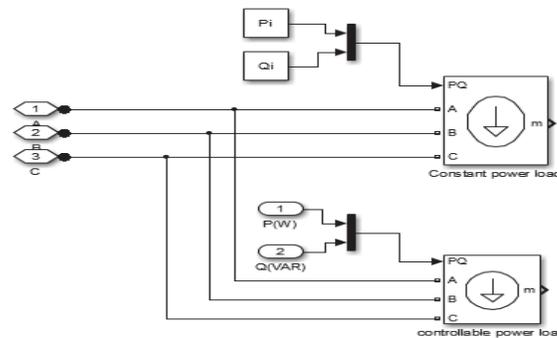
**Figure 4. Controllable load model**
