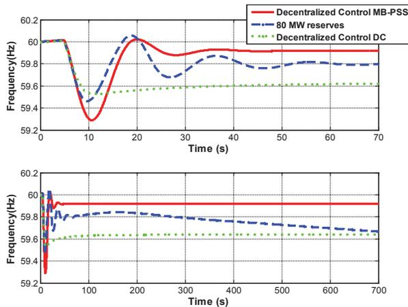
**Figure 11: System frequency with decentralized control and no reserve/80 MW spinning reserves**
