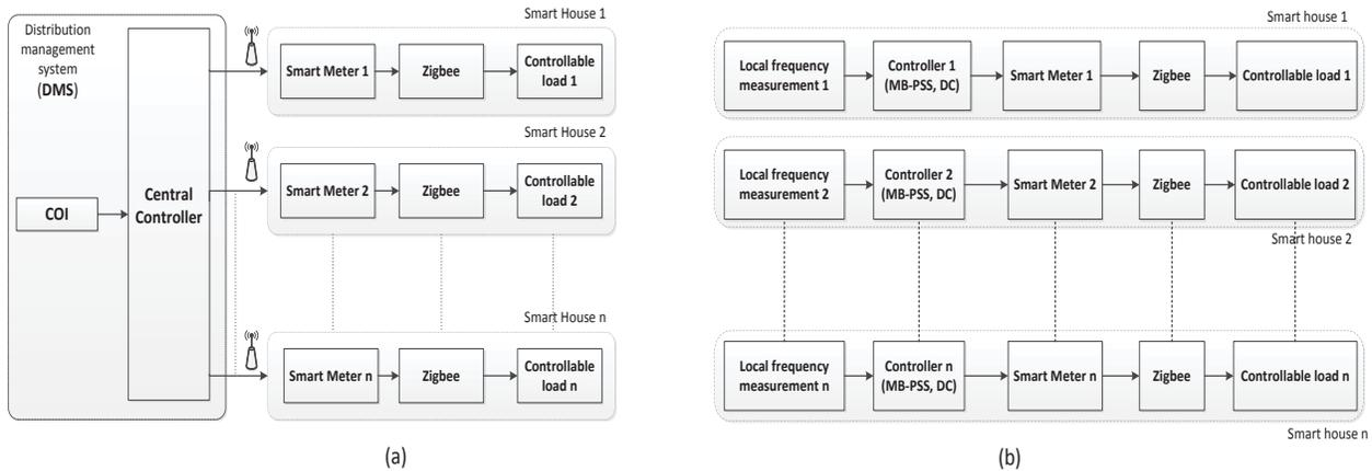
Figure 1. Overview diagram of centralized mode (a) and decentralized mode (b)
