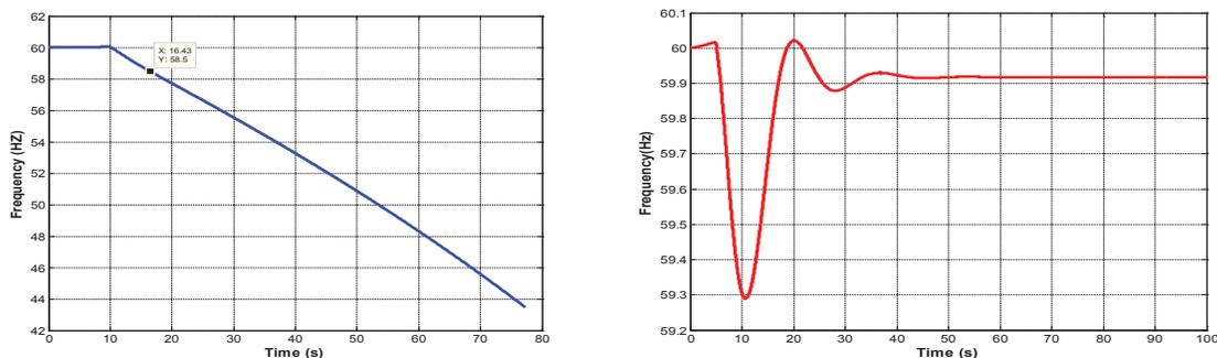
**Figure 7: System frequency with no control and no reserve (left) and with 80 MW of spinning reserves and no control (right)**
