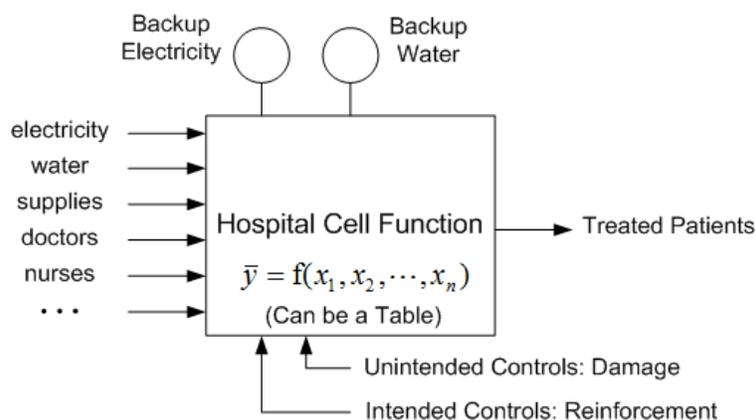
Figure 2. A conceptual i2Sim cell model [6].
