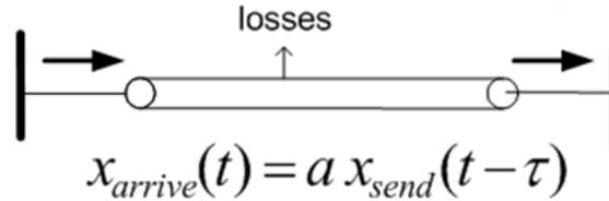
Figure 3. A conceptual i2Sim channel model [6].
