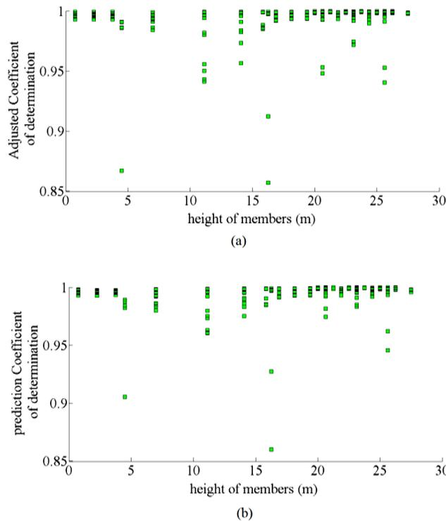
**Figure 3. (a) Adjusted coefficient of determination and (b) Prediction coefficient of determination for all members of tower 2**
