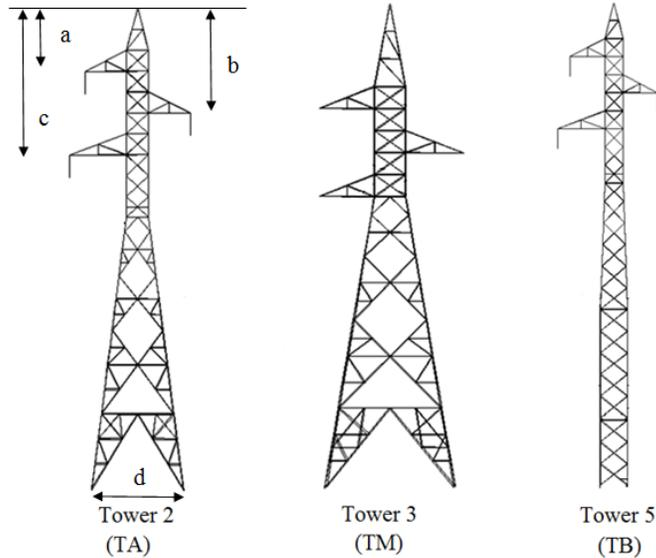
Figure 2. The configuration of tower types within the line.
