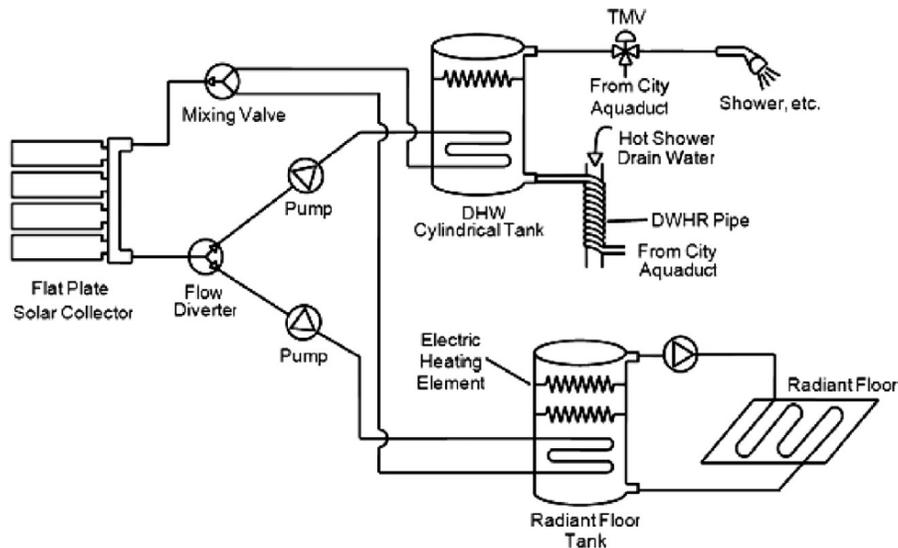
Figure 1. Schematic diagram of the residential solar combisystem [12]
