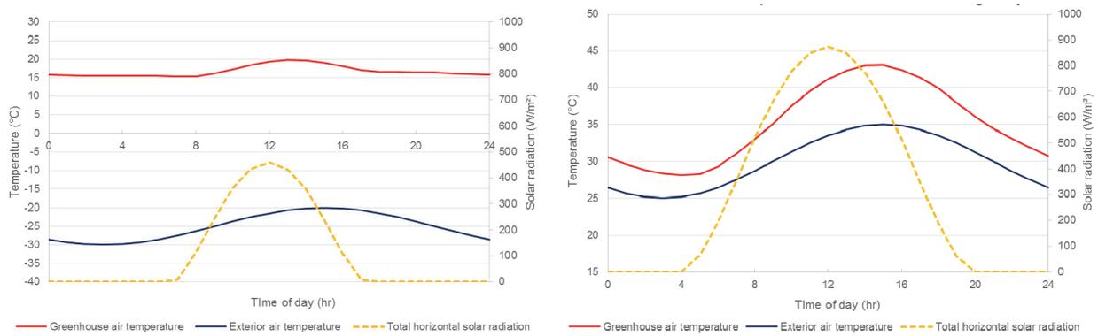
Figure 5. Daily greenhouse temperature during peak winter (left) and summer (right) design conditions.
