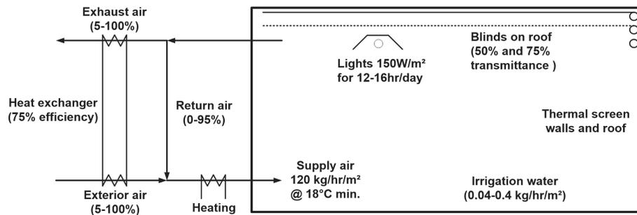
Figure 4. Greenhouse climate control details.
