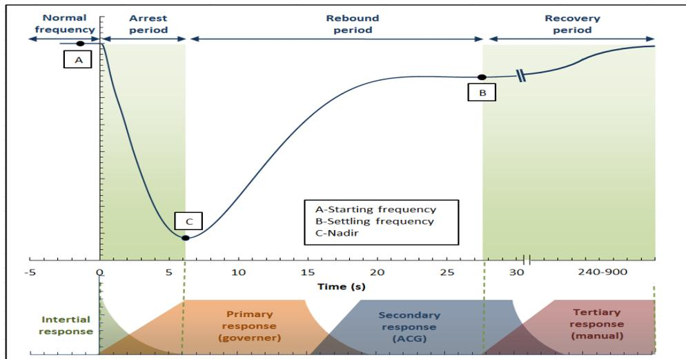
Figure 1: Illustrative frequency response after the loss of a generation unit
