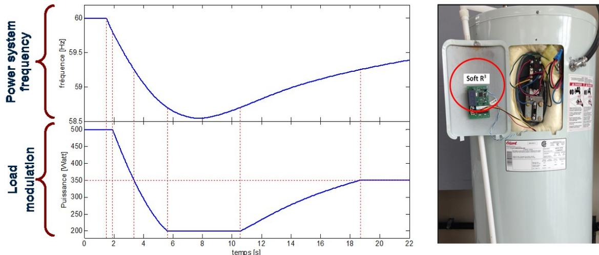
Figure 4: Frequency variation and load modulation for a Soft-R3 installed on a domestic water heater
