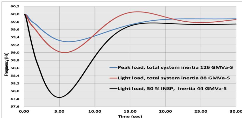
Figure 2: Comparison of frequency response for loss of 1000 MW in peak load and light load conditions
