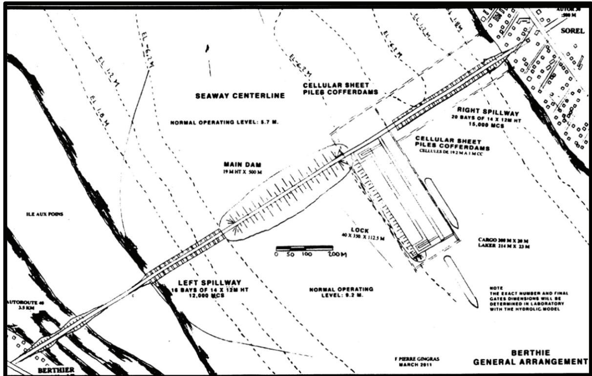
Figure 3 Control dam of Sorel-Berthier - General layout
